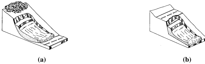
Figure 13. Location of slide mass relative to roadway: (a) slide above roadway and (b) slide below roadway (Hopkins et al. 1988).
